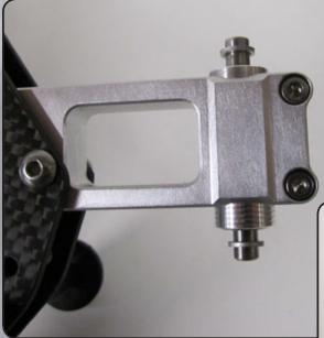
We can start our presentation by looking at the front-wheels: the pin of the steering pivot has been changed with an updated version which is lighter and which looks better than the previous one.
