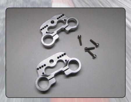
The steering mounts of the forks are from our own production and are characterised by the distance of the forks' pipes which is close to the hole of the pin of the steering pivot. This features gives to bike a better stability when riding fast bends as well as more steering corner when riding slow bends.
