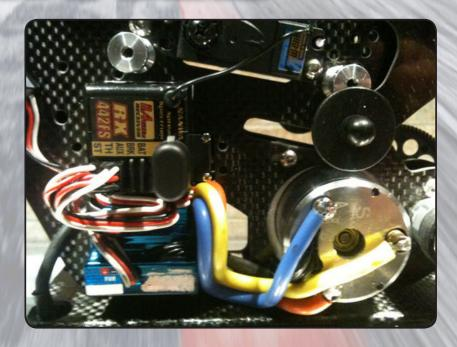
The position of both ESC and servo brake has been changed in order to reach a better balancing of the base towards the low part and in order to let the brake wire slides much more easier than before.
