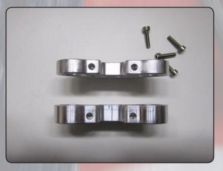
The steering mounts are supplied in two different thicknesses the low one is in fact thicker than the up in order to make the fork stronger.
