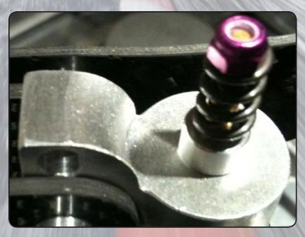
The rear shock absorber is made in an exclusive way and allowed us to reduce weight of about 55 gr so that the rear part of the bike is now really closed to that of real bikes. Its position which is almost perpendicular to asphalt let the shock absorber grants an optimal traction when exiting from the bend
