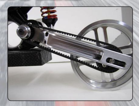
The transmission is reduced in its diameters allows to step on the gas while turning reducing at the same time the sideslip and making the bike easy to drive when exiting from the bend.
